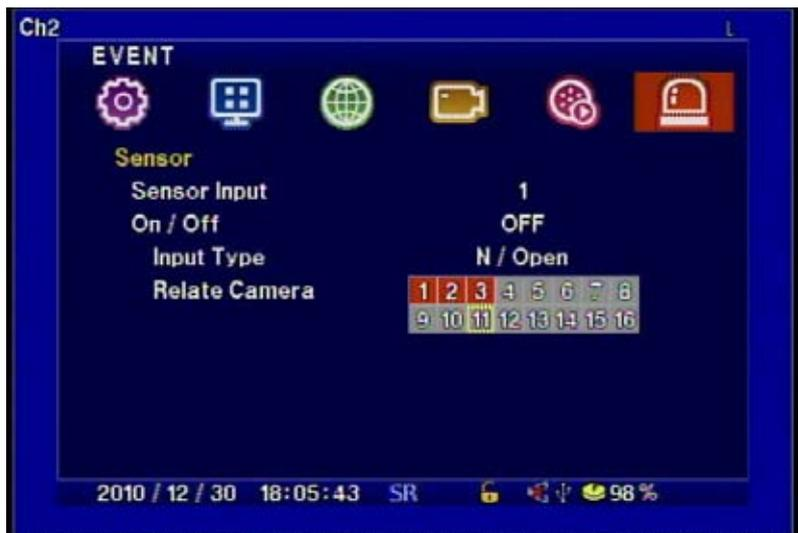
[1] Sensor Input : Select the sensor input channel.
