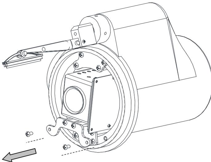
4. Loosen the two screws and then apart the camera module out of the Housing. Then the rear connector is taken out as showing the above figure.
