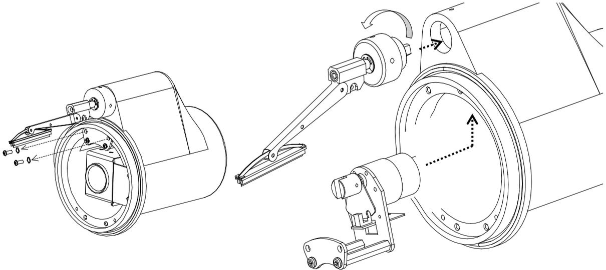
**1. Loosen the two screws on the bracket.**
