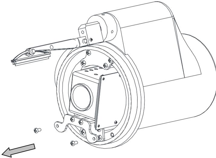
**1. Loosen the two screws and then part the camera module out of the Housing. Then the rear connector is taken out as showing the above figure.**
