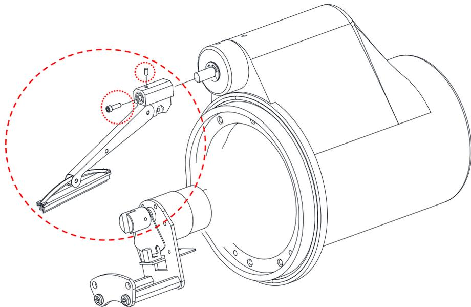
**2. Loosen the Hexagon socket head screws and depart the wiper bar from the wiper head. It can be changed as the expendable supplies.**
