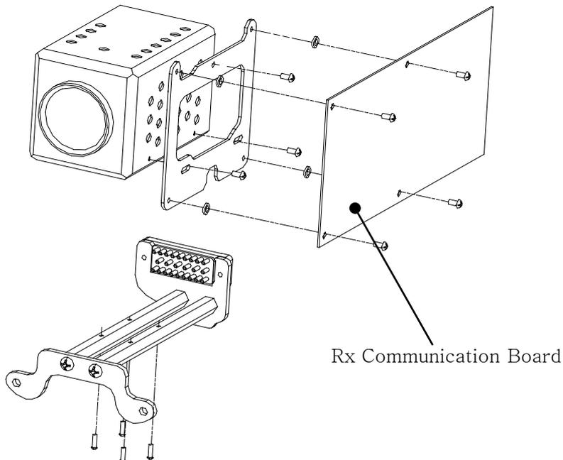
**2. Loosen the screws such as the picture and part the Rx communication Board from the assembly.**
